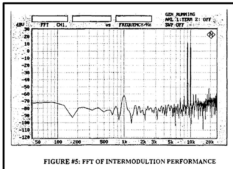
Figure 5: Intermodulation Performance
